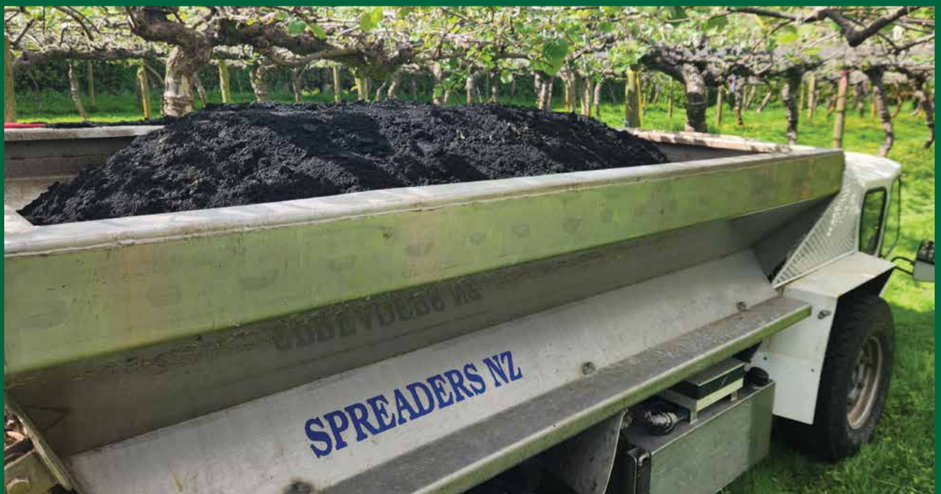
Biochar is a charcoal-like substance formed by burning biomass (such as forestry waste) at high temperatures without the presence of oxygen.
